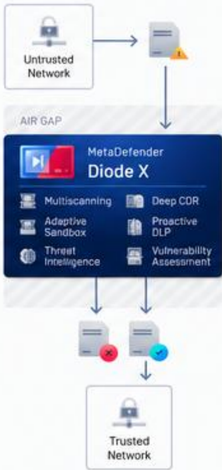
One way data transfer with additional file sanitization by MetaDefender Core
